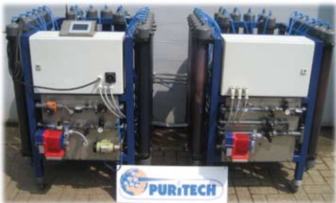
Figure 1. Continuous counter-current demineralization unit
